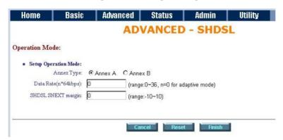
The screen will prompt the parameters that will be written in machine. Be sure to confirm the modified parameters before rebooting and activating these changes in GRT-101/GRT-401.
